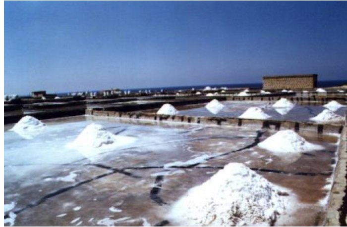
Fig 5. Salt exploitation through solar evaporation.
